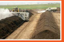
fter your green cart is emptied, the yard debris and food scraps are hauled to a commercial composting facility operated by A1 Organics in Keenesburg, Colorado. At this facility, the organic material is ground into fine pieces by an industrial grinder. Smaller pieces help to speed up the decomposition time. The material is then placed into long narrow piles called "windrows" that are turned on a regular basis to enhance aeration.
